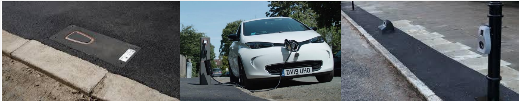
A pop-up charger when recessed, and when in use.
